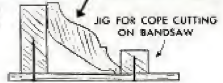
Moldings can be mitered and coped on power tools, using the circular saw for the miter cut and the bandsaw and simple jig for the cope cut
